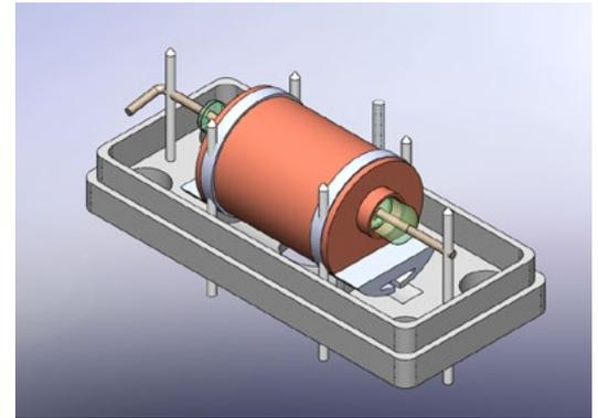
3D printed relay component
