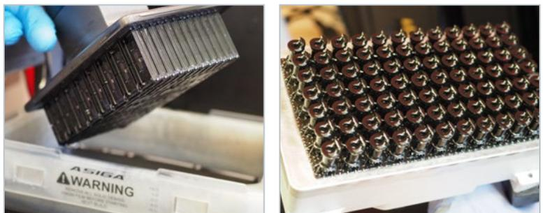
3D Printed Relay Components
