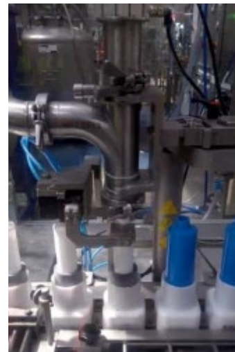
50 ml and 250 ml bottles being filled in the same production run
