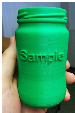
Packaging prototype 3D printed with FDM (photo courtesy Get3DSmart)
