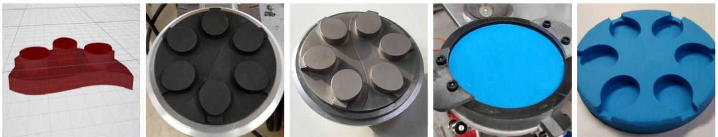
Transition from 3D printing and nickel plating to final silicone mold
