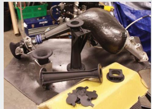
Air intake with 3D printed parts
