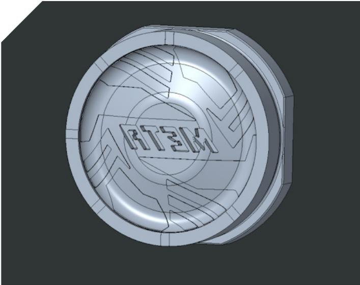
Above / CAD image of the mold cavity
