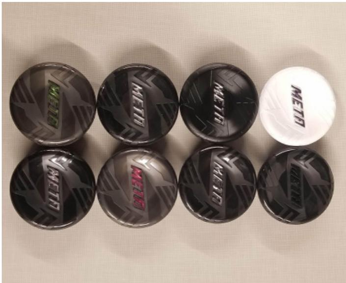
*Above / DeMarini Sports needed a way to quickly evaluate and test a range of polymers and part designs without tying up its production toolmakers. The solution? 3D printed plastic injection molds from Fortify.*
