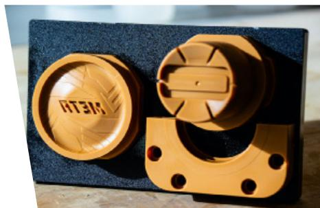
Fortify proposed that DeMarini use the FLUX ONE to produce its prototype tooling. The FLUX ONE utilizes Continuous Kinetic Mixing (CKM) to prevent the clumping and sedimentation that otherwise occurs when printing the highly viscous, ceramic fiber-filled resins needed for injection molding tools. Further, the system's Fluxprint technology serves to align those fibers, reinforcing critical areas, increasing mold strength, and extending tool life 10X to 100X more than competing 3D printers.
